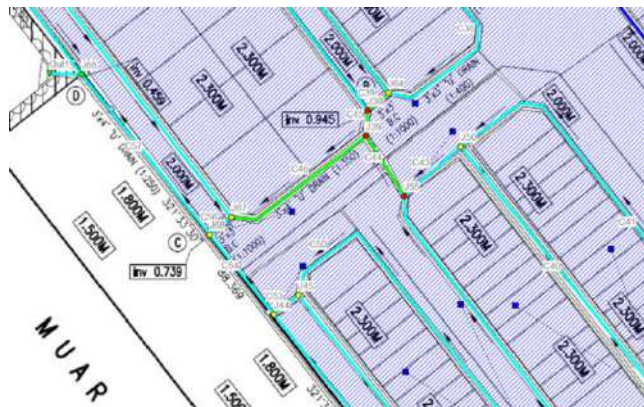
Figure 8: Bottleneck Stormwater Mitigation Path
