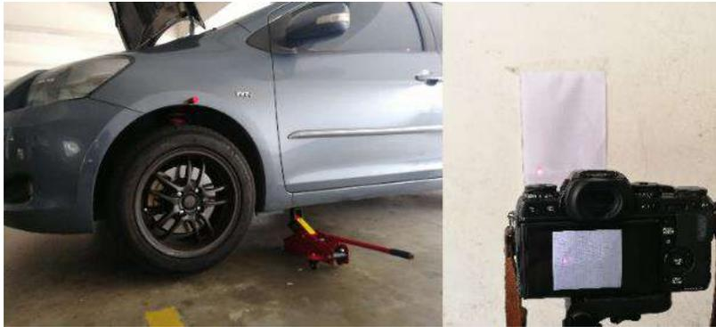
Figure 10: Actual set-up static drop test
