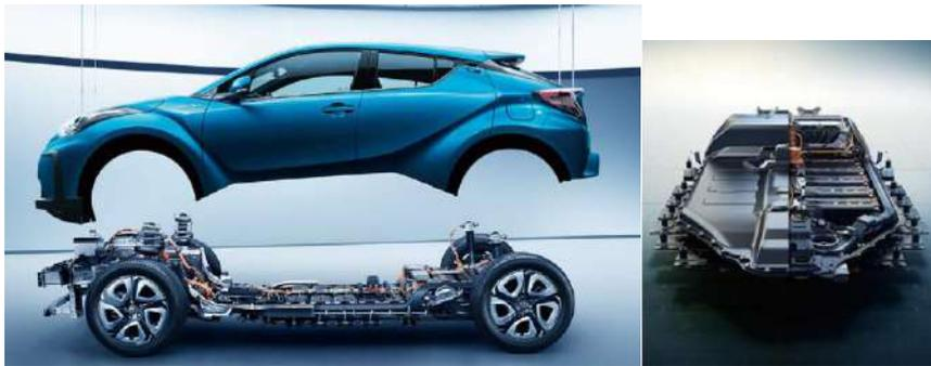
**Figure 3:** Chassis structure and battery module of Toyota C-HR EV
