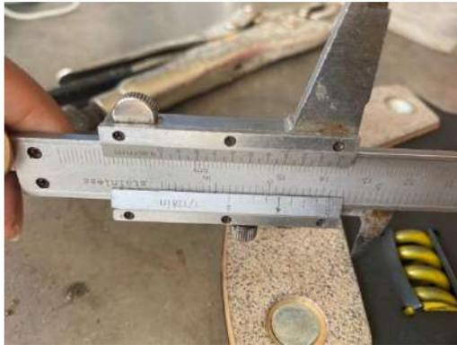
**Figure 5:** Clutch Plate Inner Diameter (Aftermarket)
