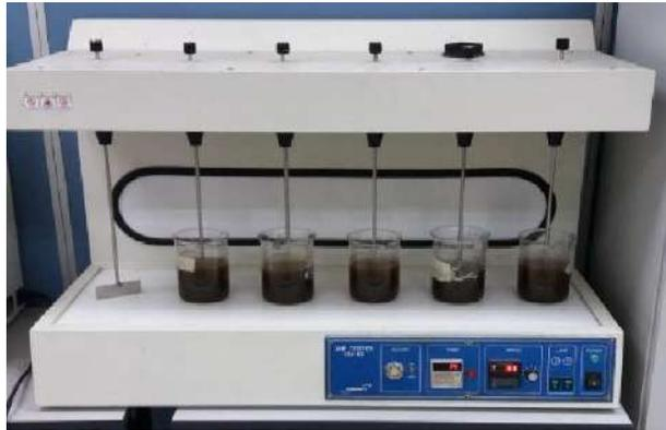
**Figure 4:** Mixing using jar test
