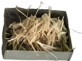
**Figure 2:** Sugarcane bagasse fibre
