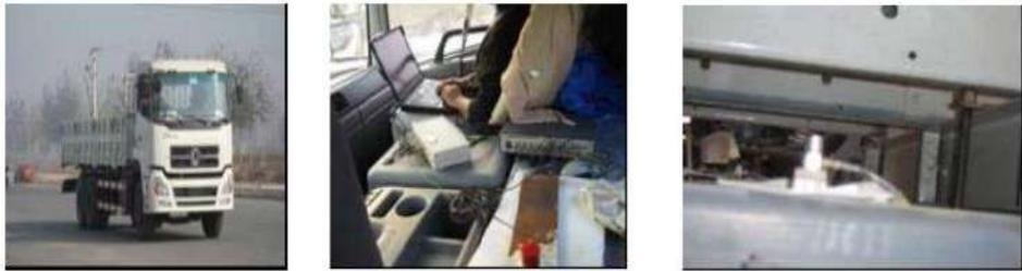
(a) The vehicle in the field test      (b) Acceleration transducer on cab seat      (c) Acceleration transducer on vehicle body
