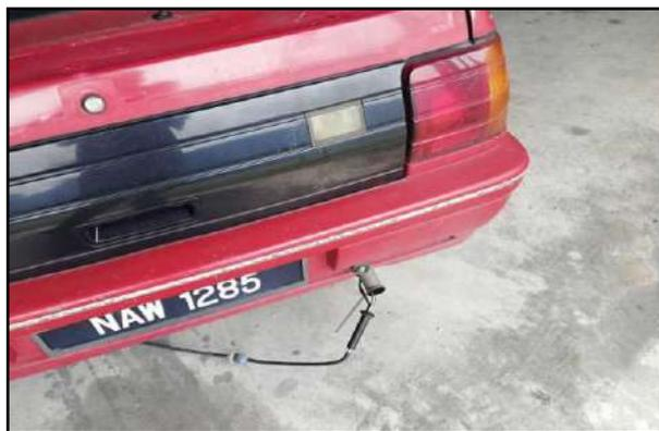
**Figure 4:** Exhaust Gas Analyzer Installed at the exhaust pipe.
