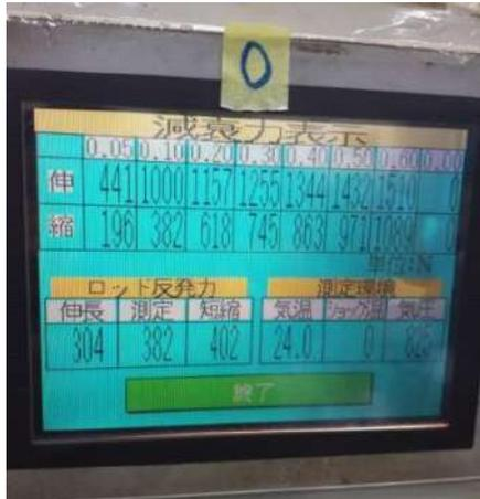
**Figure 8:** Sample result of shock absorber tester on the monitoring display
