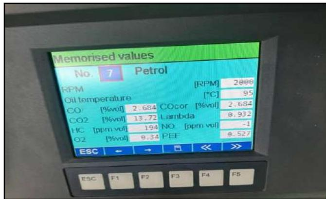
**Figure 5:** Output Exhaust Gas Emission
