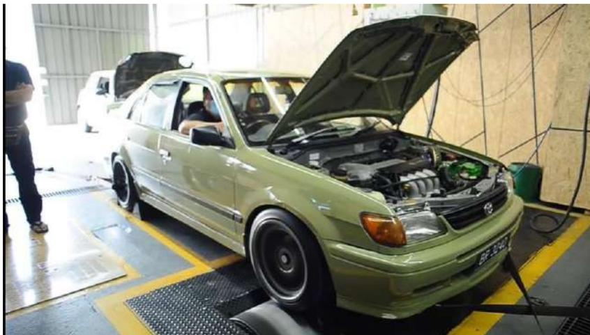
**Figure 2:** Vehicle Strapped on Chassis Dynamometer
