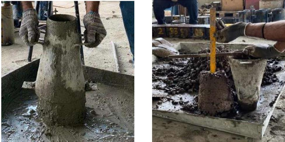
**Figure 3:** Slump test setup and procedure.
