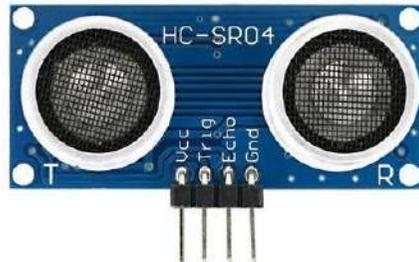
**Figure 1.3:** Ultrasonic sensor
