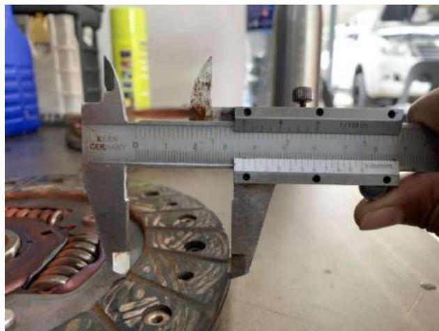
**Figure 4: Clutch Plate Contact Surface Area (Conventional)**
