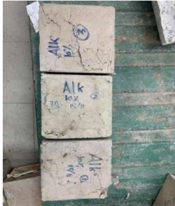
**Figure 5:** The damaged concrete cube samples after the compression test.
