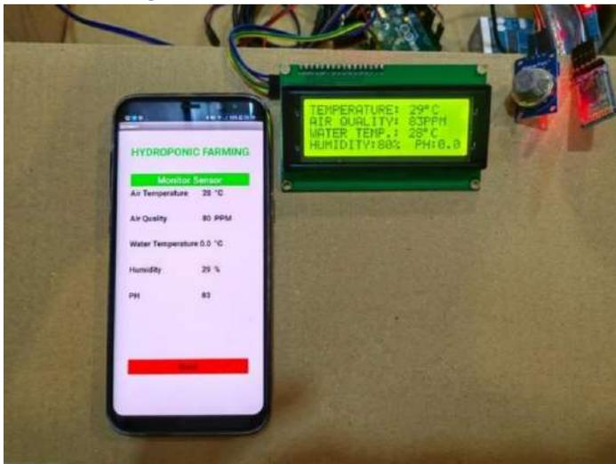
**Figure 16:** Monitoring of temperature, air quality, water temperature, humidity and pH value.
