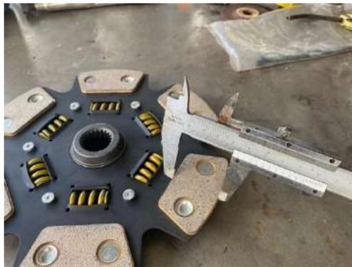
**Figure 6:** Clutch Plate Contact Surface Area (Aftermarket)
