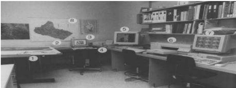
**Figure 2 :** Typical GIS Laboratory with Components: (1)Scanner; (2)Digitizing Table; (3)AutoCAD/ArchiCAD Personal Computer; (4)Tape Driver; (5)Workstation; (6)Colour Printer; (7)PCARC/INFO Personal Computer; (8)Typical Drainage Map. (De Mesnard, 2017)
