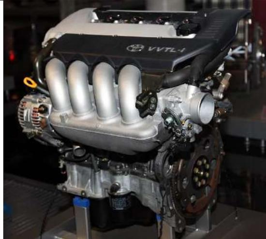
**Figure 1(a):** Toyota Soluna and **1(b)** 2ZZ-GE Engine Overall View ([www.toyota.co.jp](http://www.toyota.co.jp))
