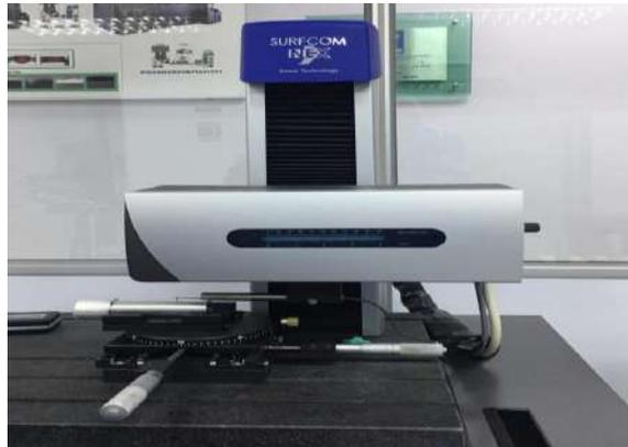
**Figure 4:** Surfcom Nex for Ra Measurement
