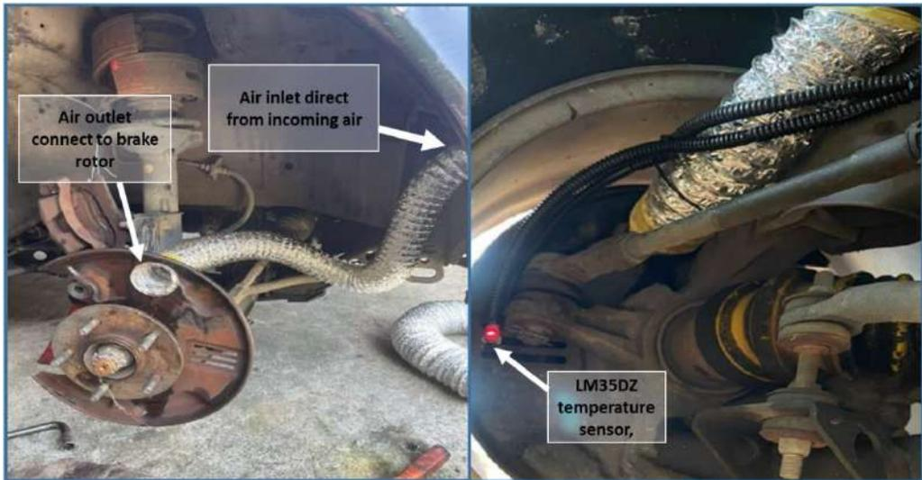
**Figure 1** (a) Hose installation (b) Temperature sensor location
