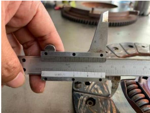
**Figure 3: Clutch Plate Inner Diameter (Conventional)**
